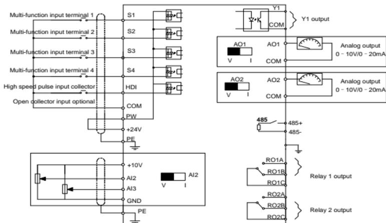
Fig 3.6 Wiring of control circuit of G200UL-01 versions
