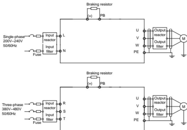
Fig 3.3 Connection diagram of main circuit
