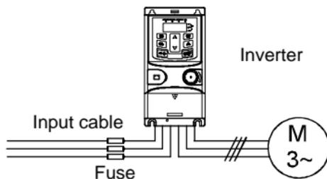
Fig 3.12 Fuse configuration
