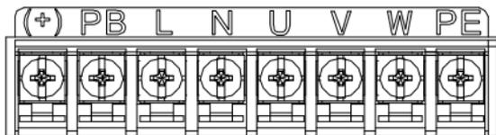
Fig 3.4 1PH terminals of main circuit
