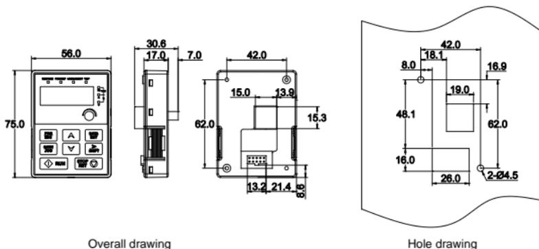
The external keypad can be mounted on the installation bracket and the bracket is optional.
