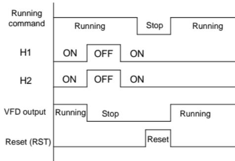
2. When the hundreds of [P11.16](#) is set to 1, the STO alarm will be unlocked
