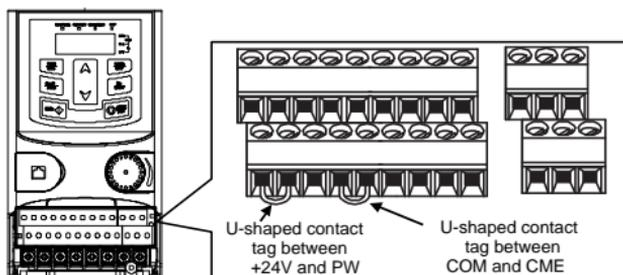
Fig 3.9.1 U-shaped contact tag of G200UL-01 versions
