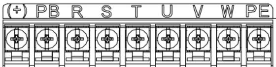
Fig 3.5 3PH terminals of main circuit
